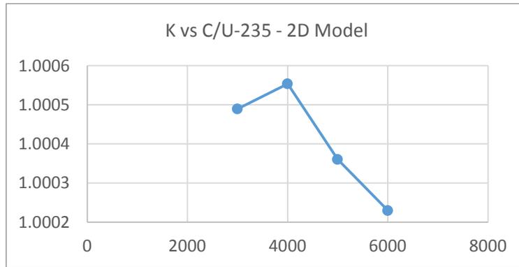
**Figure 5: K-eff vs. C/U-235 ratio (2D Model)**
