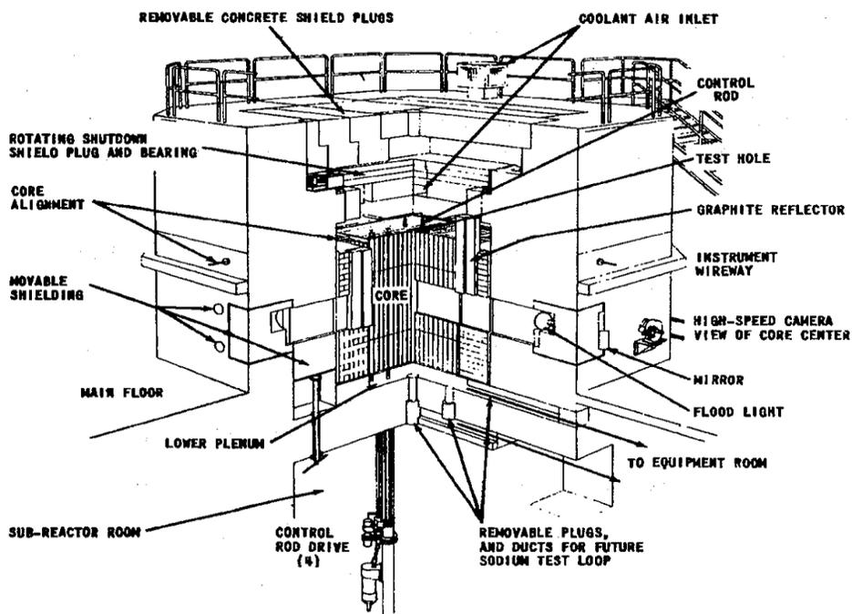
Figure 1: Perspective view of the TREAT Reactor
