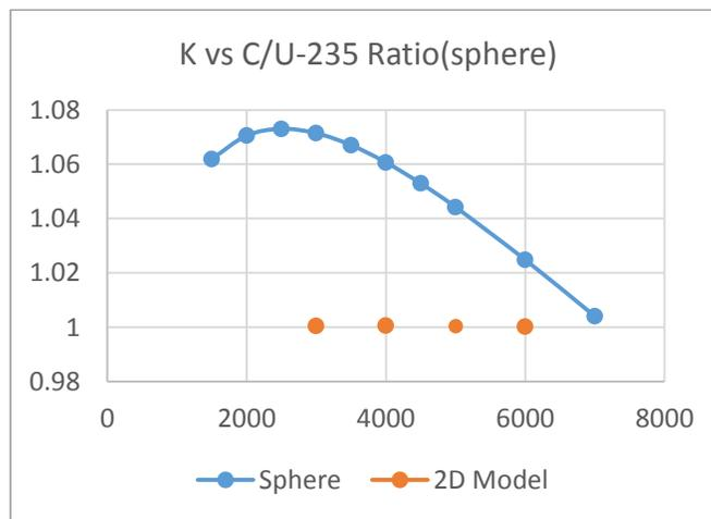
**Figure 4: K-eff vs. C/U-235 ratio (Spherical Model)**
