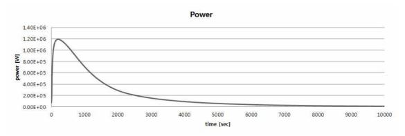
Figure 4. Power level of core after RIA
