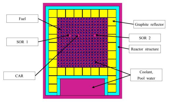
Figure 1. Core Model of H-LPRR
