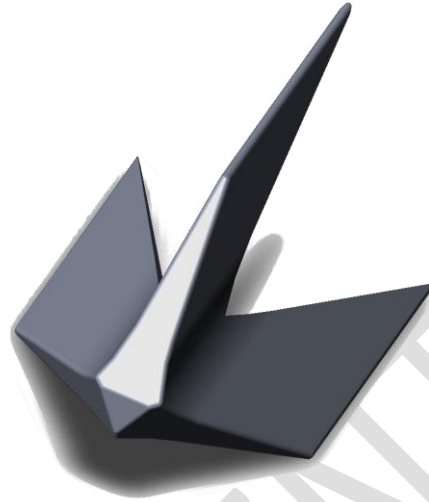
8. Lower Fuel Element Fin Geometry
