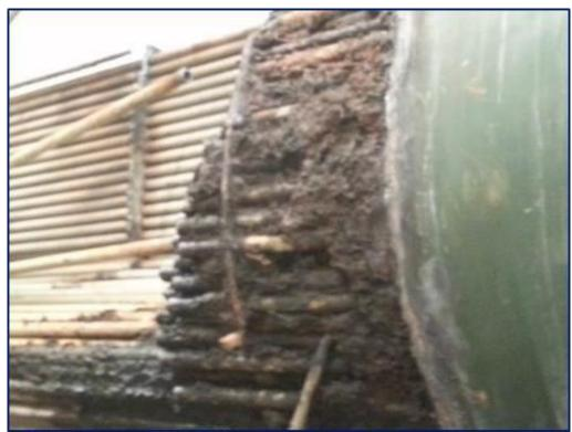
Figure 3: Old Heat Exchanger Corrosion
