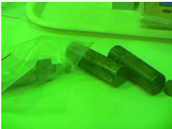
Element w/ No Cladding
