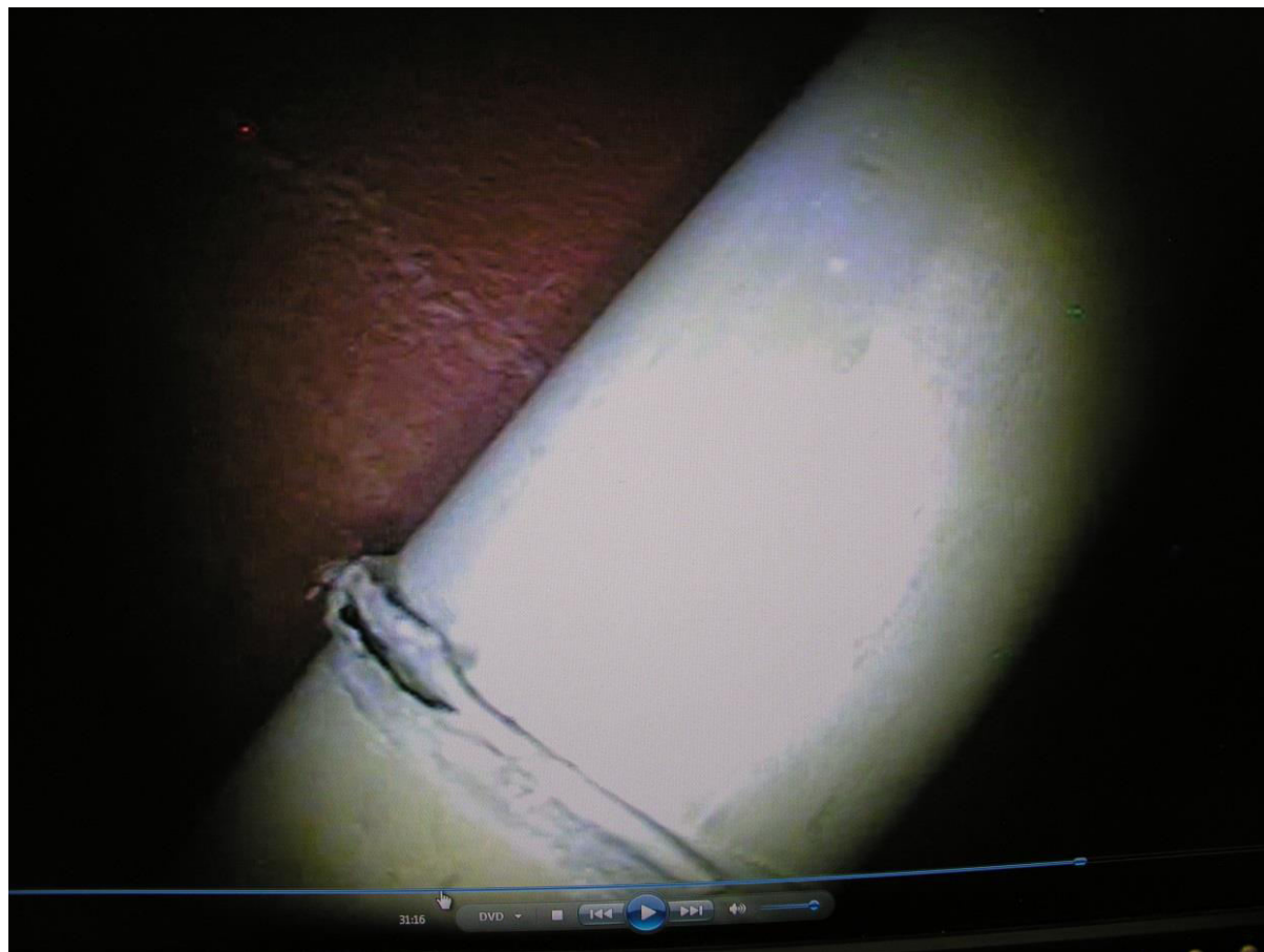
Al-Clad TRIGA Element w/ Breached Cladding
