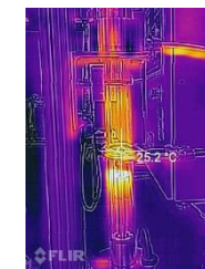
ATF-2 SQT instruments pin assembly and thermal imaging during brazing process at HTTL
