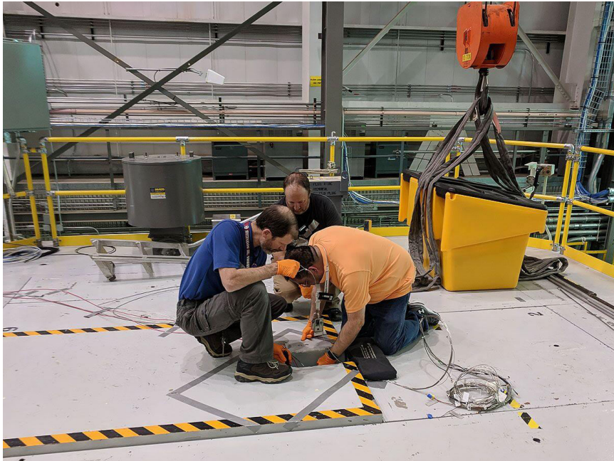
Loading Instrumentation Assembly into TREAT M8CAL Core
