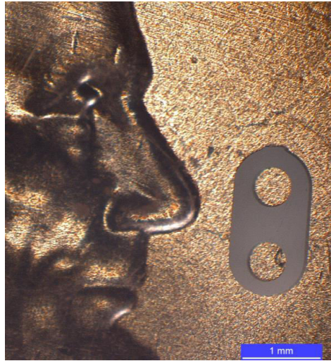
The small size of the MPFD sensor allows for insertion into a flux wire port 1
