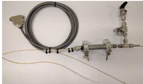
5-node common cathode MPFD with 10 ft extension wiring, gas purge/fill pre-assembly and electronics feedthrough 1
