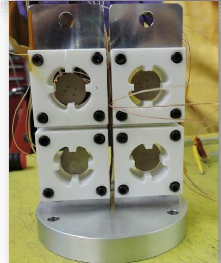
Setup of test sample stakes from earlier DU tests
