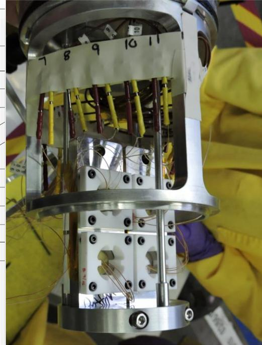
Strain relief of TCs following assembly of the Bi and DU samples
