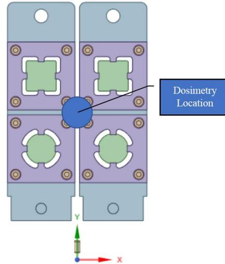
2D Representation of 2 Sample Steaks and (Purple) MACOR holders to hold sample coupons with dosimetry packet in center
