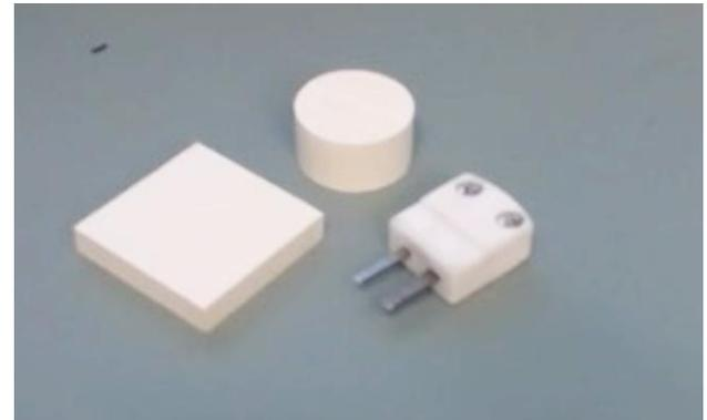
Boron nitride samples: PCBN1000 (square) and AX05 (round) for shielding and ceramic pin connector for future development
