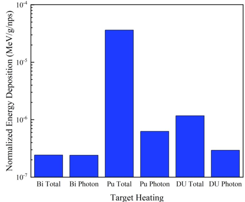
MCNP6.2 Produced Energy Deposition Estimates for ACRR Pulse Operation in Bi, Pu, and DU
