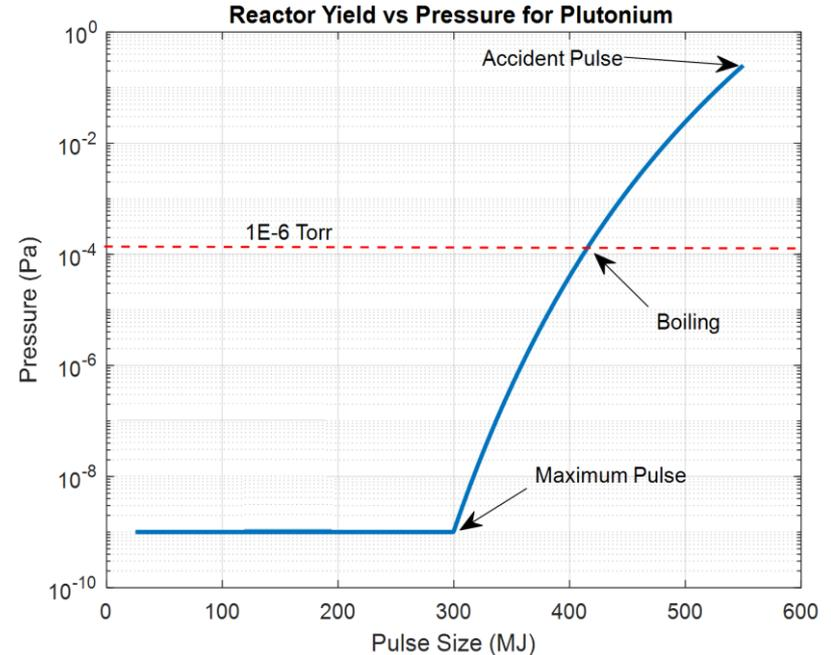
Pressure vs. Reactor Yield Analysis for Maximum Pulse (300 MJ) and Accident Pulse (550 MJ) for Plutonium Sample in ACRR
