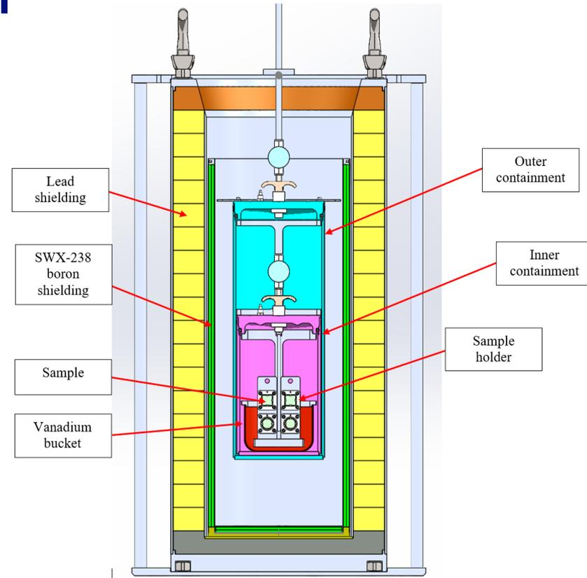
CAD Cutaway of Experimental Package
