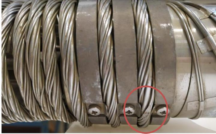
**Figure 11: Indication of wear on the wiring**
