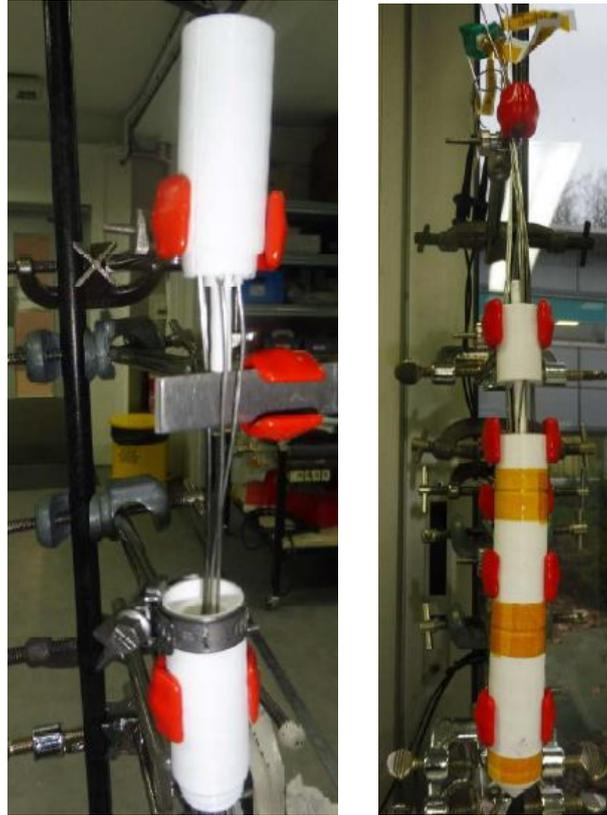
**Figure 8: Assembly of the 3D model printed calorimeter**
