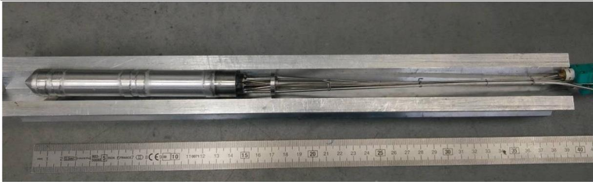
**Figure 6: Calorimeter mock-up before and after assembly**
