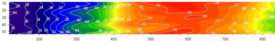
Figure 5: the calculated burn-up distribution in a high density silicide fuel plate, irradiated in the FUTURE basket for 88 days.
