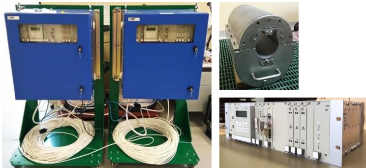
Figure 5: Boron Concentration Monitor (from left, clockwise): Signal processing units in cabinet; detection unit; DBK 250 signal processing modules in 19" rack
