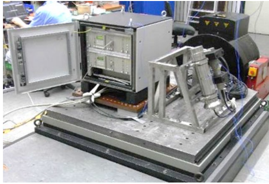
Figure 4: Seismic test set-up for cabinet with two signal processing units DAK 250 i and two NaI scintillation detectors SG 65 M (inside thermal shield) plus SG 66 R on support
