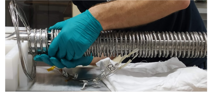
Sensor cables formed in spiral
