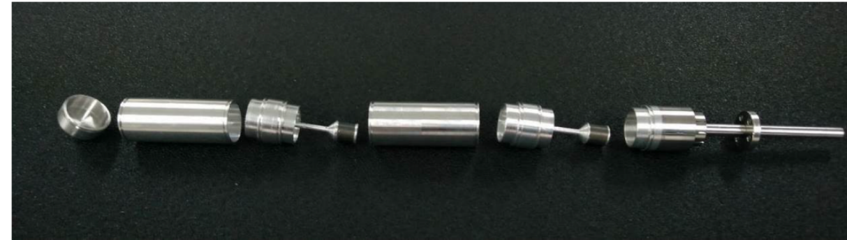
Calorimeter mock-up before and after assembly
