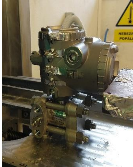
Fig.6: The irradiation chamber with alanine detectors placed on the tested sensor from both sides and the same levels
