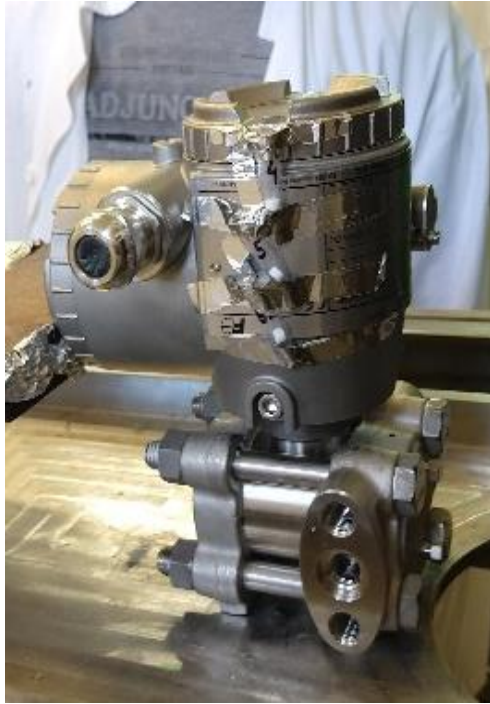
Fig.6: The irradiation chamber with alanine detectors placed on the tested sensor from both sides and the same levels
