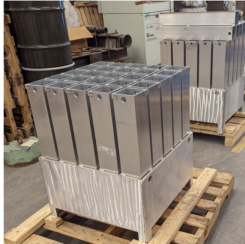
Three 5x5 fuel storage racks were fabricated by MIT central machine shop. The rack design was modified based on the HEU spent fuel storage rack design. One fuel rack will be used for fresh LEU fuel elements.
