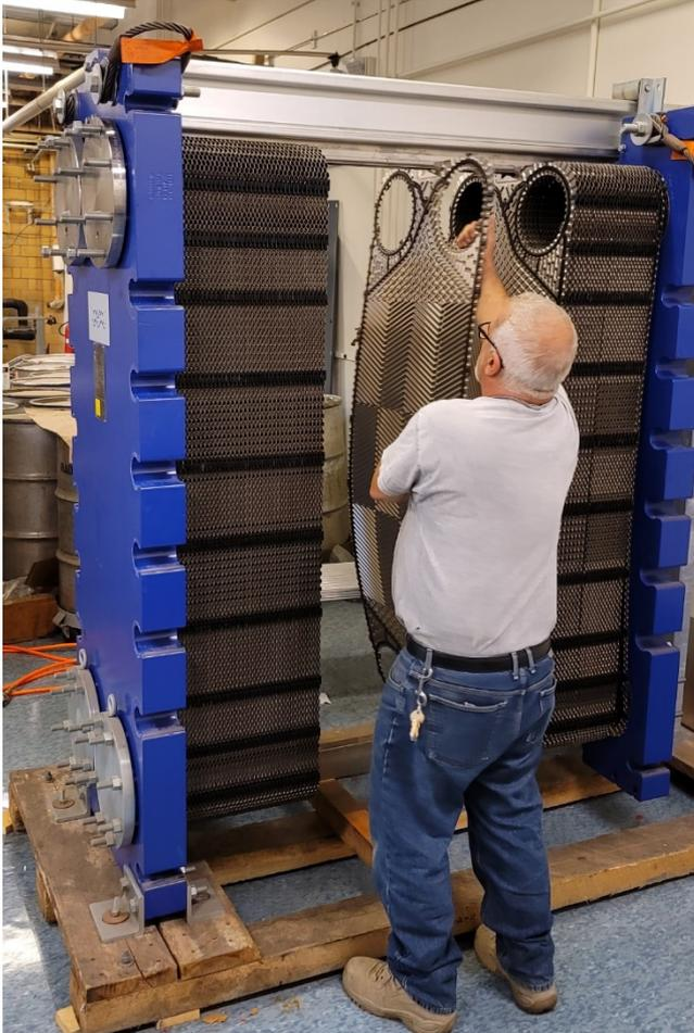
Plate-and-Frame heat exchanger
