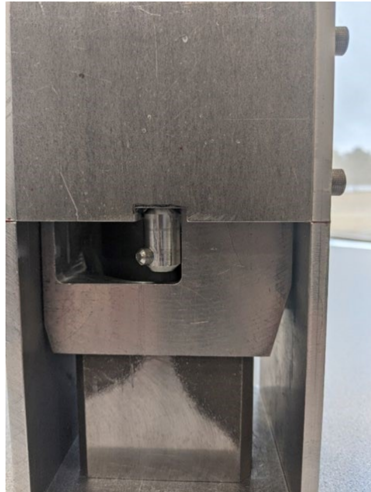
Fuel element head latched into a mockup of the upper grid plate.
