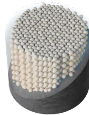
Illustration of FCM fuel pellet interior
