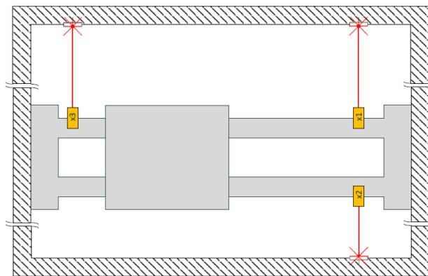
Figure 3: Laser System for Position Detection
