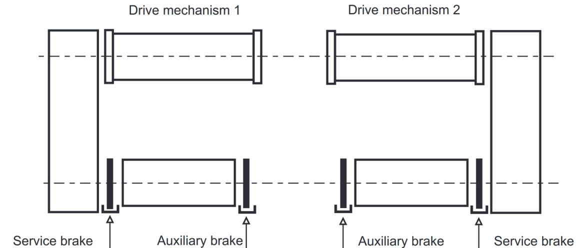
Figure 4: Schematic view of 20 t lifting unit and brakes
