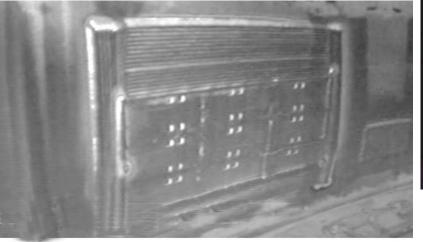
1250 cm<sup>2</sup> repair area3x3 array of structural platesNine unique welding processes
