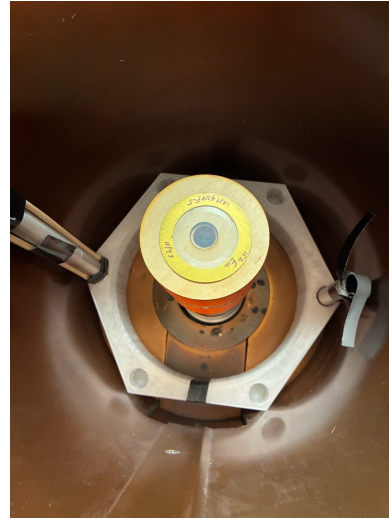
Figures 3 & 4: Europium sample within the HPGe detector and its Lead shielding
