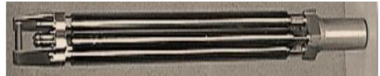
TRIGA 4 Element Fuel Cluster (MTR Conversion)
