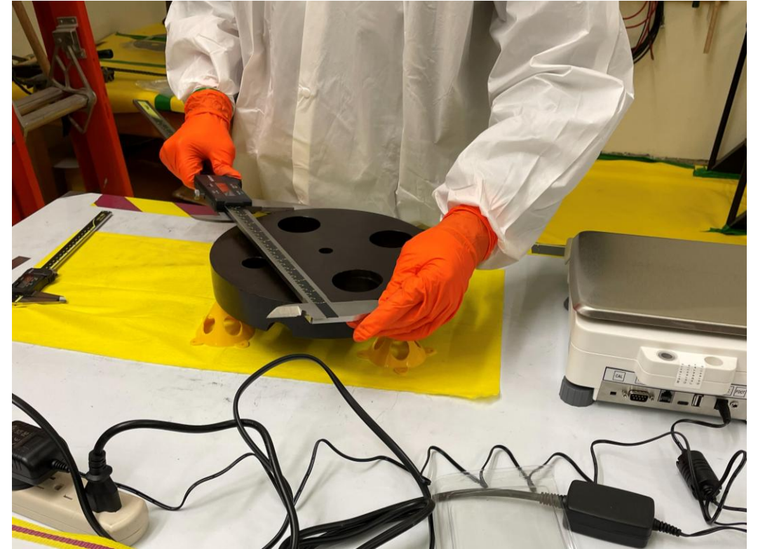
Fuel disk diameter measurement
