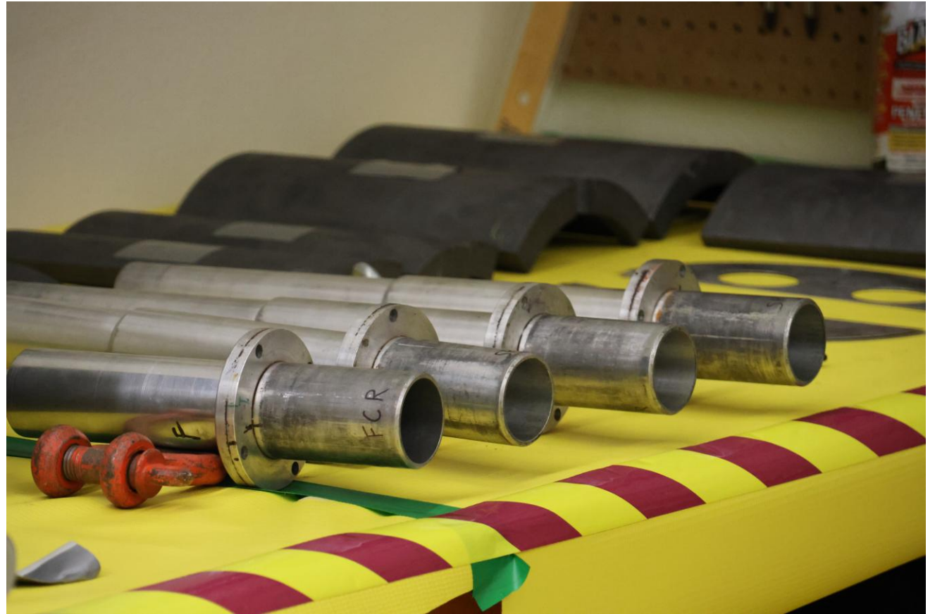
Control rod thimbles and graphite shells
