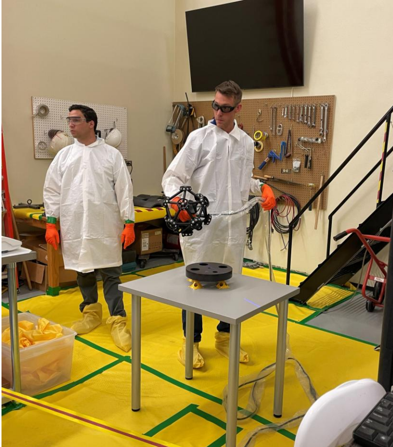
Using a Coordinate Measuring Machine to model a fuel disk
