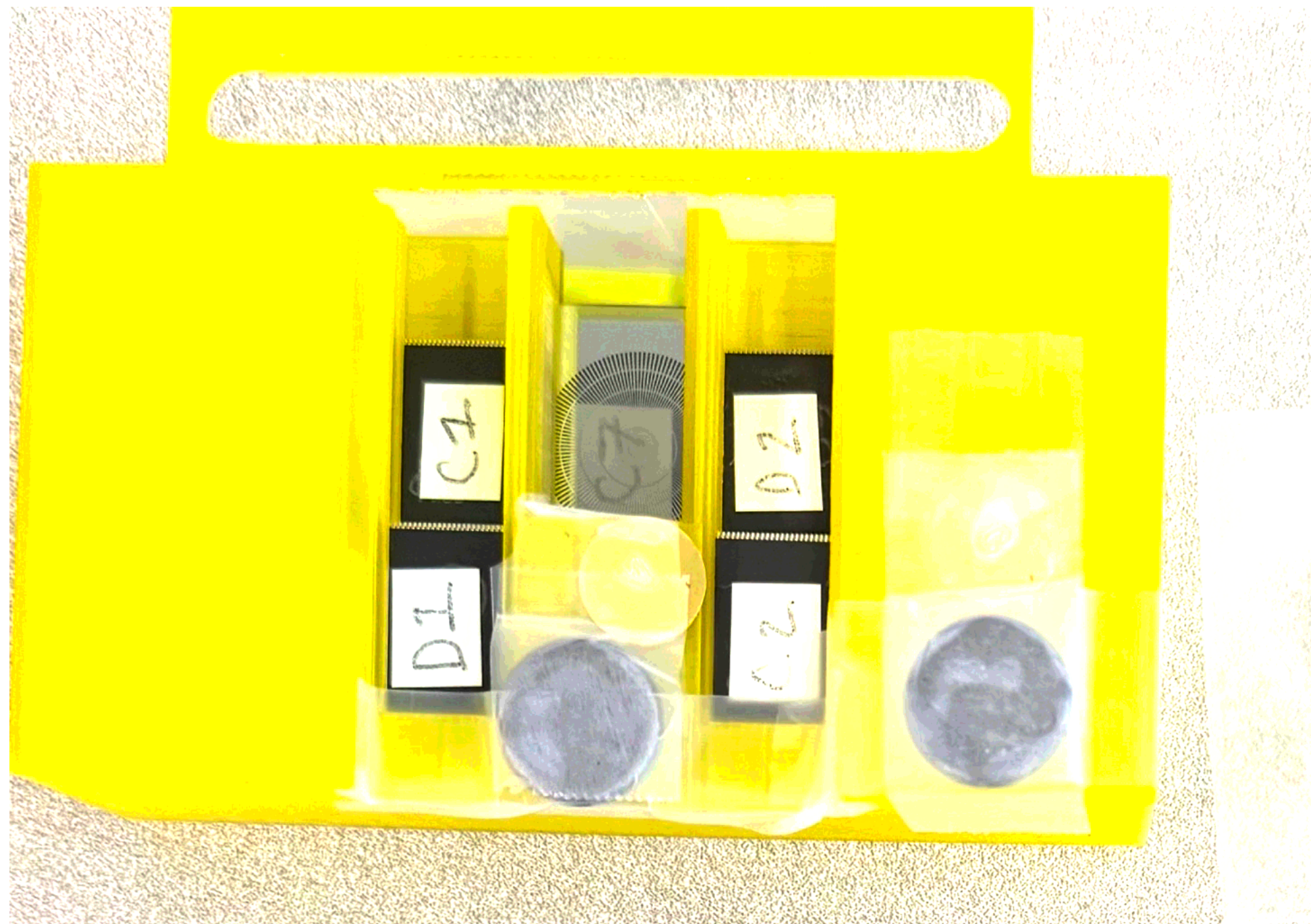
Fig 7: 3D printed device holder (yellow), NISoC prototypes (black, labeled), gold foils & cadmium covered gold foils.
