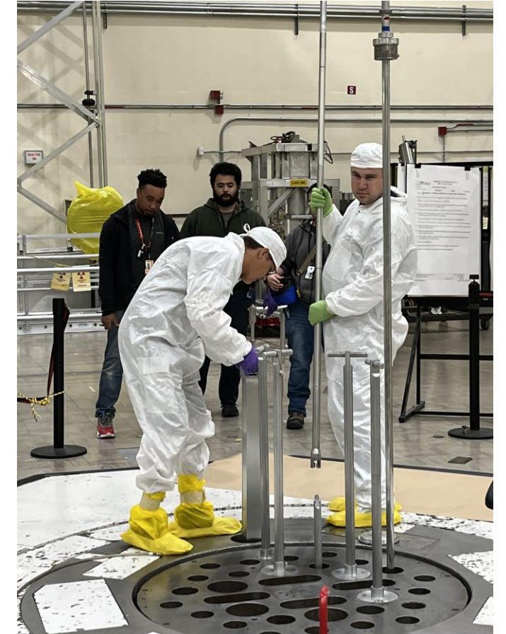
Refueling in preparation for reactor restart
