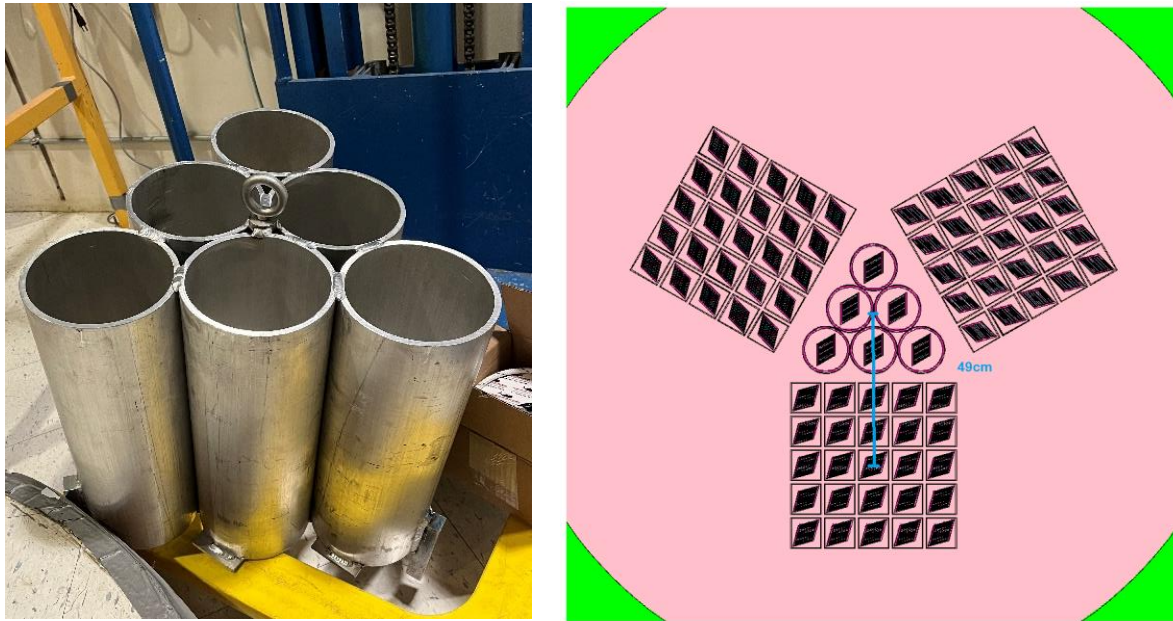
Figure 4: Temporary storage rack after component welding but before final de-burring and cleaning for install into SFP (left). Full SFP racks under most conservative conditions, with temporary Al6061 storage rack in the center. 81 total HEU elements modelled, 10% cadmium mass assumed in permanent rack liners (right).
