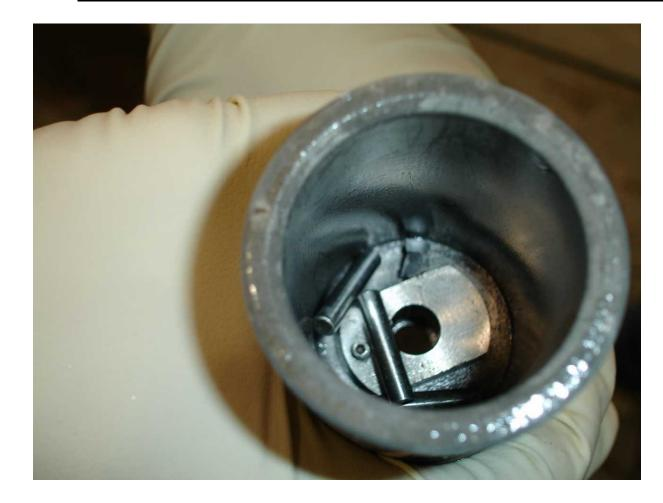
TR C: 3 steel pins from retainer
